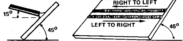
Figure 8-22. Horizontal Weld Beads - Inclined Plate
