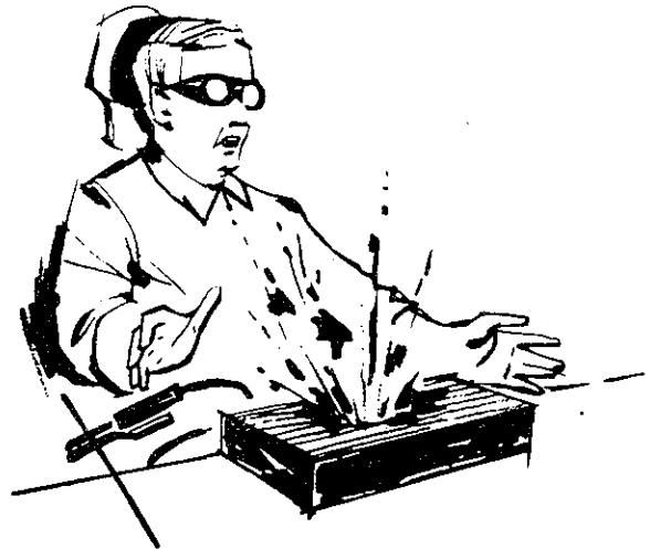
Figure 1-6. Don't weld on hollow (cored) castings
