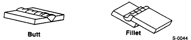
Figure 12-1. Flat Position Welds
