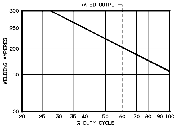
40% Duty Cycle At 250 Amperes
