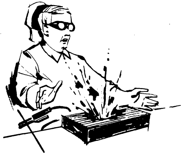
Figure 1-6. Don't weld on hollow (cored) castings
