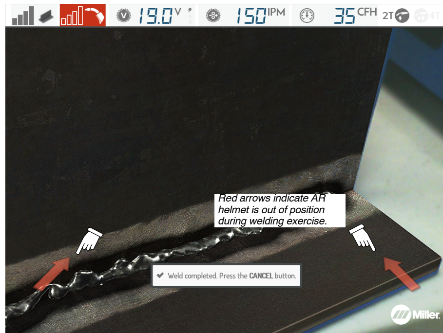
Figure 7-16. Arrows Indicating Error In Helmet Position
