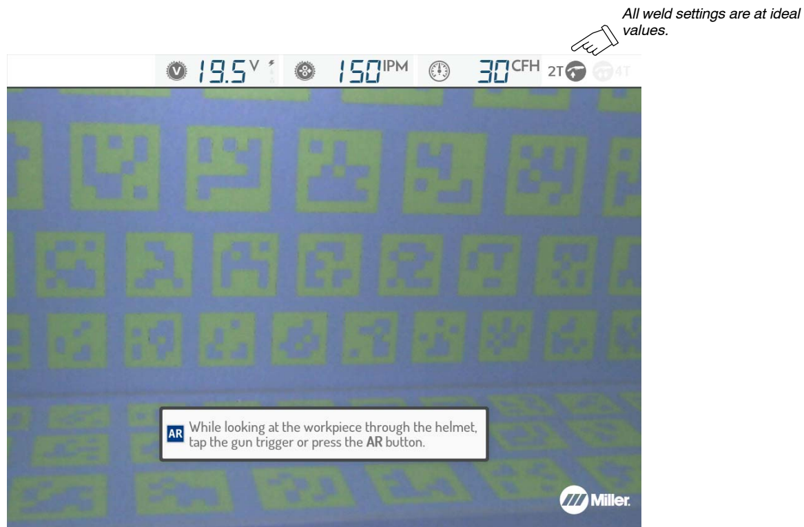
Figure 7-11. Example Of Acceptable Weld Settings
