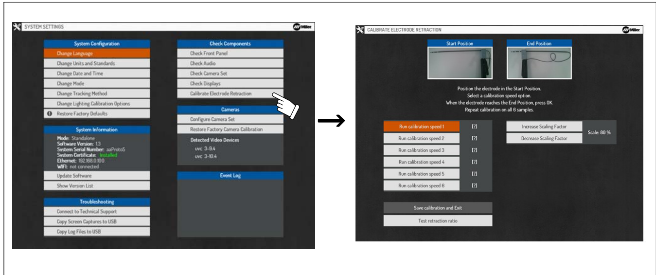
Figure 8-10. Calibrating Stick Electrode
