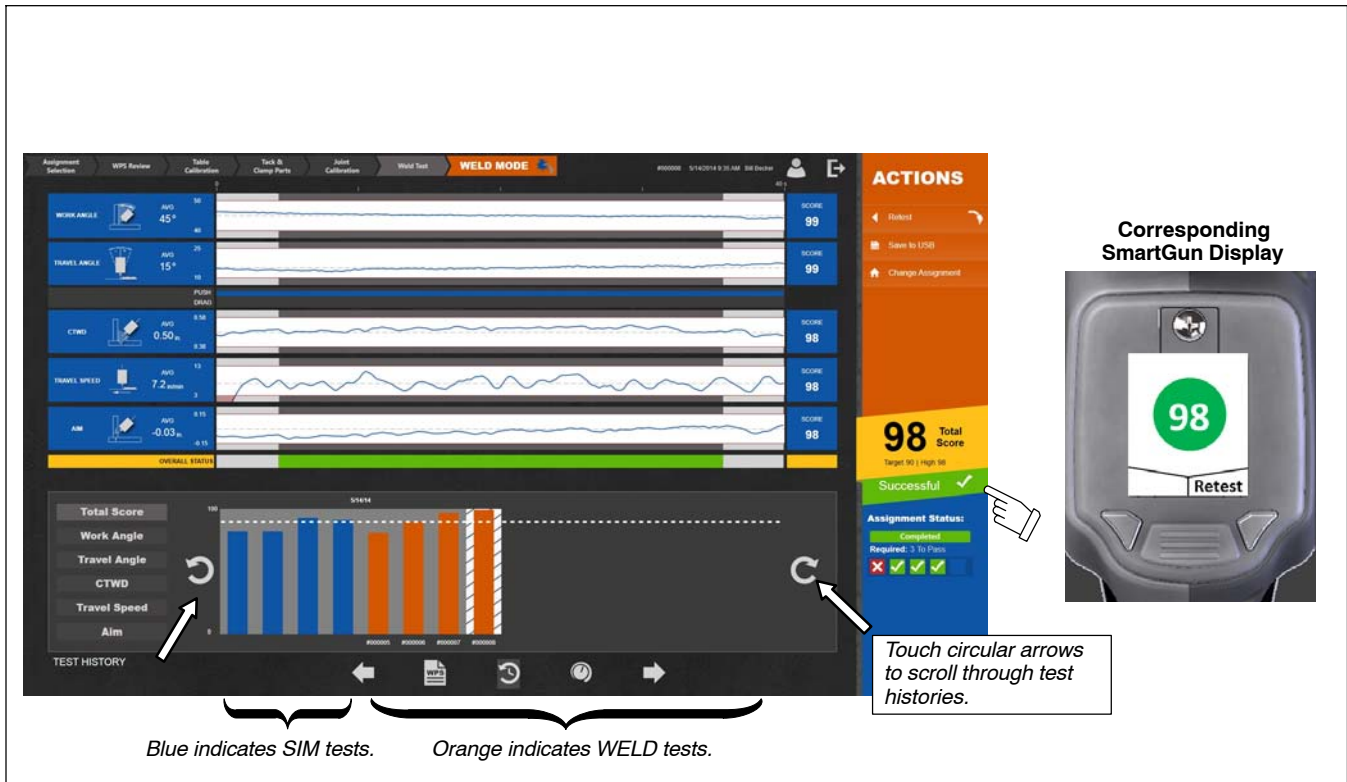
Figure 7-21. Successfully Completing The Welding Assignment
