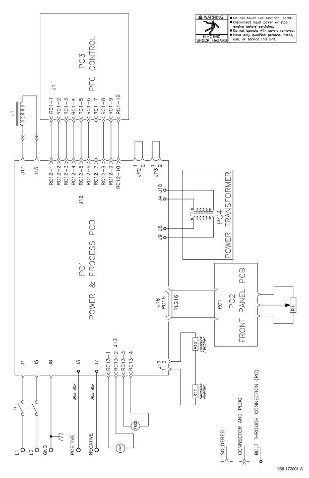
Figure 7-3. Circuit Diagram For Si 160 PFC
