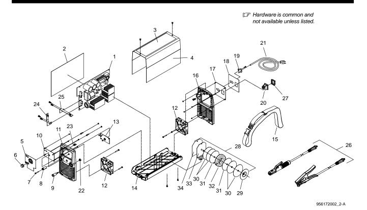
Figure 10-1. Main Assembly For Si 160 PFC
