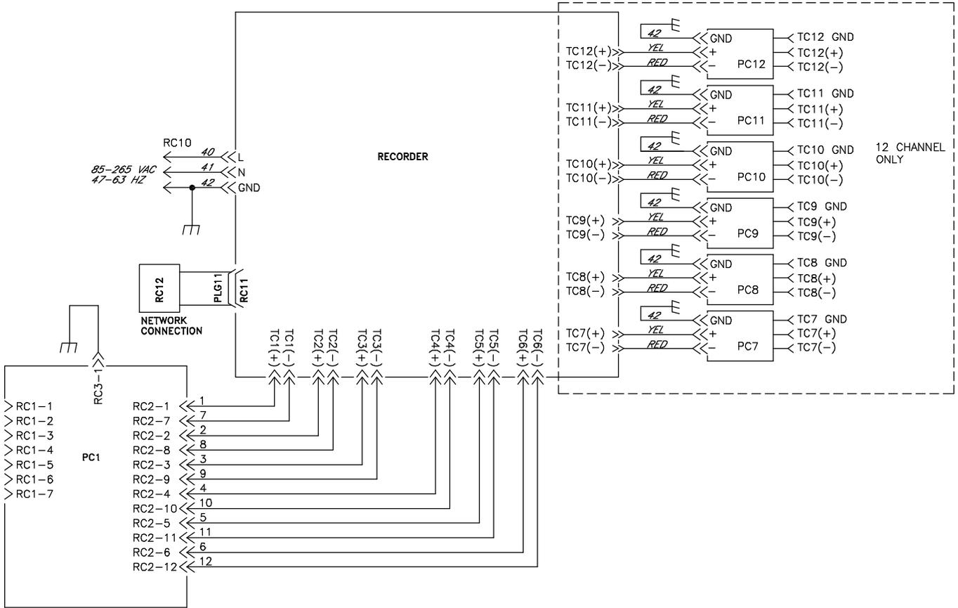
Figure 8-1. Circuit Diagram For Digital Recorder
