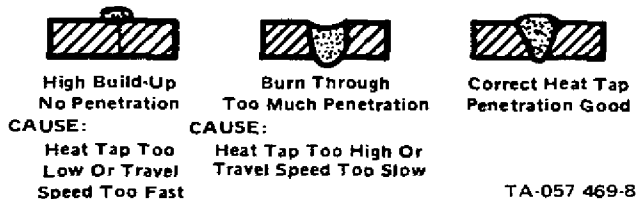
Figure 4-5. Cross Cut View of Various Welds
