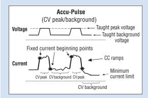
The Accu-Pulse process allows for precise control of the pulse arc. Accu-Pulse provides optimum molten puddle control and has power to increase wire feed speeds and deposition 20 to 25 percent in many applications. In most cases, slightly different ratios of gas mixtures will perform well using a similar program and adjusting arc length or the appropriate arc control for the selected process. Contact Miller for more information on less common materials and gas combinations.
