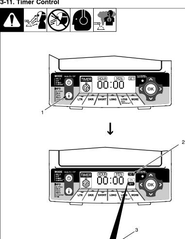
The Timer emits an audible signal and flashes the Grind mode light to alert the operator after a specific period of time has elapsed.
