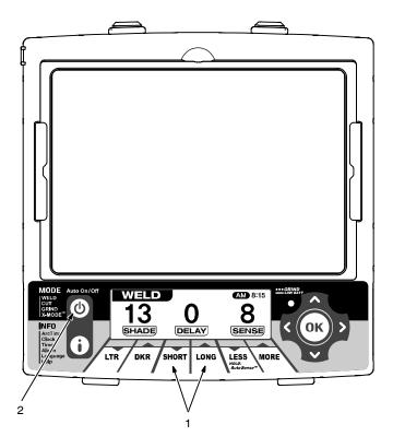
Lens Delay Adjustment Buttons
