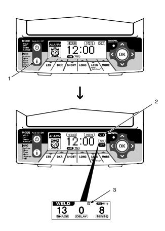
The Alarm emits an audible signal and flashes the Grind mode light to alert the operator at a specific time.
