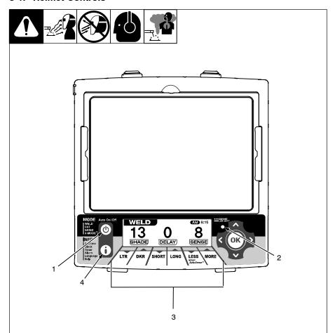
The auto-darkening lens turns on (darkens) automatically when welding begins and turns off when welding stops.
