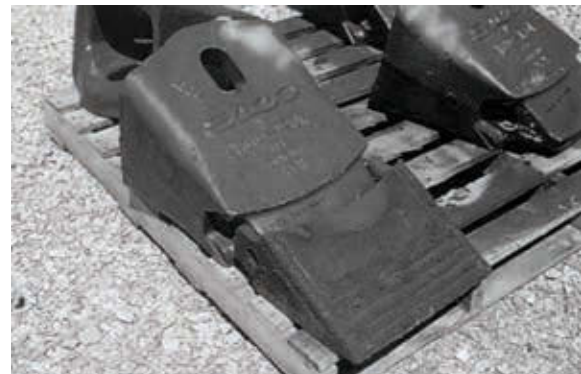
Figure 7 – OVERLAY - Replacement Dragline Bucket Tooth Hardfaced As New Equipment.
