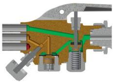
**Closed Flo-Trol valve.** If there is insufficient oxygen, the oxygen is unable to overcome the force of the Flo-Trol spring, stopping the flow of preheat oxygen or mixed gas travelling back to the system from a starved tip.
