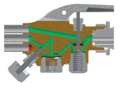
**Open Flo-Trol valve.** When the oxygen supply pressure is able to overcome the force of the spring, the Flo-Trol valve opens, allowing the free flow of preheat oxygen.
