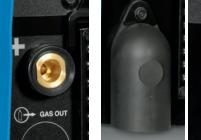
Tweco® versus studs. The XMT 350 is equipped with Tweco-style weld connections (left) while the XMT 450 (see page 1) is equipped with studs (right) for ring-lug output connections.
