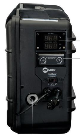
Digital meters with SunVision™ technology display voltage and wire speed, and amperage if desired. Meters can be seen clearly even in direct sunlight.
