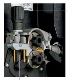
**Ultra-low drag inlet guide pins** make loading the wire easy and do not deform the wire on the way into the drive rolls. Simply thread the wire through the pins and into drive rolls.
