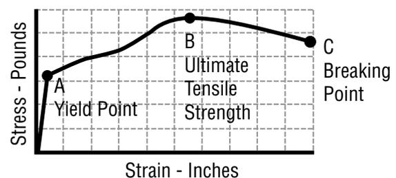
Figure 3 – Stress Strain Curve
