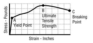
Figure 3 – Stress Strain Curve
