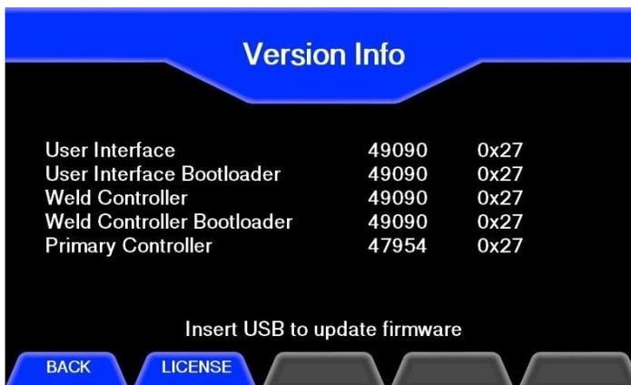
3. If the machine powers up with an error, power down the machine. Power it up again; press and hold down the fourth button from the left below the LCD screen during the power up sequence until the Version Info Screen appears.
