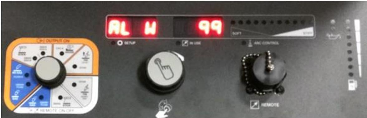
6. Once the update is complete, the welder will resume normal operation and the system will be ready to weld. At this point it is safe to remove the USB thumb drive and begin using the machine again
