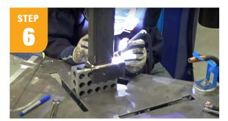
Because my rear frame is smaller, I am using the 2"  $\times$  3" square tubing and attaching it to the saddle.
