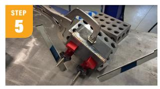
Frame mounts for the rear of my car are not as wide or thick as those for the front, so they will be built differently. I used the same 3/16" flat plate and TIG welded the corners. Since I had a hole already in the frame, I am attaching it using two 3/8" rivet nuts on each side. You can do that or attach it just like we did in step 4.
