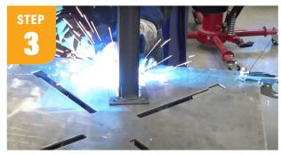
For the front frames, weld the castor mounting plates to the 2-1/2" square extension tubes using the Multimatic 220 AC/DC in Auto-Set™ mode for 3/16". I only welded a 1-1/2" to 2" weld on each side.
