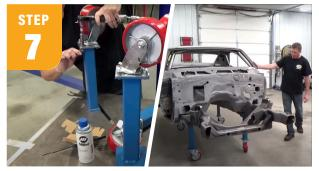
Assemble the four castors to the four mounting plates, and then attach the rolling car stands to the car frame.
