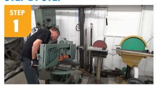
Determine the height you want the rolling jack stands to be off the ground, and cut the extension tubing and castor-mounting pads. My extension tubing is 14-1/2" and the flat plate for mounting the pads is 4" x 4-1/2".
