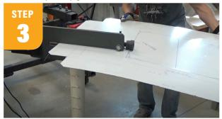
Using a bead roller with step die, in the center of the sheet, put an offset facing inside. This will allow a little air flow behind the TV. If your bead roller is not electric, you may want another person to help.
