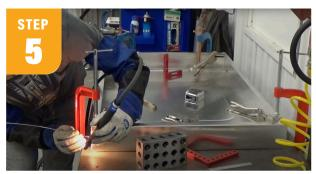
Once the bends are completed and lined up, clamp it down and tack weld the corners using your Multimatic 220 AC/DC. Start with tacking the outside and the tops, and then finish welding it all together. Remember to clean all your weld joints first using a stainless steel brush and acetone.
