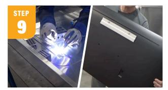
To mount the TV inside the enclosure, you can drill holes and mount it permanently or you can make an offset mount like I did using 2" strips. Run the 2" strips through your bead roller to make an offset mount. Weld one strip inside the cabinet, and bolt the other to the backside of the TV.
