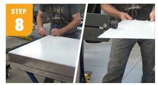
Mark and cut out a 1" x 1" notch on the front bottom panel corners using your band saw. Using a bead roller, step die a 1" lip on the two short sides and top. Then flip the panel and put 1" step roll on bottom with the notched corners so it's inverted from the other three. This will give you a lip that will slide inside the bottom of the enclosure.
