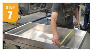
To make the front panel, measure the width and height of your enclosure. I subtracted 1/8" from each side. (Mine is 41-3/4" x 25-3/4".) Cut to size.
