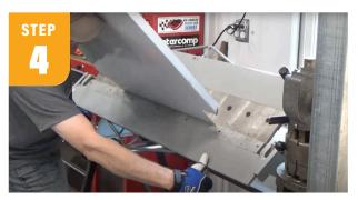
Bend the 1" lips first on your brake or metal bending tool, then the 3-1/2" bends. Remember to calculate the bend radius.
