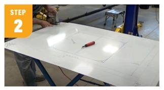
Because we will bend the sides up to enclose the TV, notch out the corners using your jigsaw and then deburr the edges.
