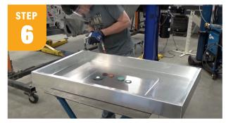
Using a small, flat sanding disc, smooth the welds on the surface of the enclosure so when you attach the front panel it will lay flat.
