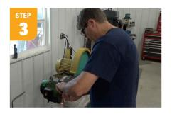
Make sure to grind and debur the sharp edges on the horseshoe pieces you've cut.
