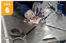
Lay out your pieces in a tree shape and tack weld them together. I used Auto-Set for the 1/8-inch setting on my machine. To produce the best welds on horseshoes, be sure to grind the mill scale off the metal.
