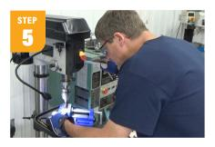
Before you weld the pieces together, drill a small hole on the end of each piece, which will allow you to hang ornaments on them. Be sure to debur the back of each drilled hole.
