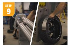
Run your shelves through slip rolls to get the radius you are looking for. If you don't have slip rolls you can use a wheel, a tire or even a metal can.
