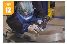
Weld your shelves to the back plate using a spool gun and starting in the middle of the shelf.
