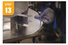
Drill holes in the back plate to hang the storage rack.
