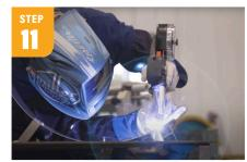
Weld your divider tab to the center and edges of your shelves. Mine are 2" from the end on the long shelf, 1.5" on the second shelf and 1" on the third, with no divider tabs on the fourth shelf.
