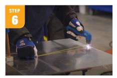
Cut the radius of the top of the back mounting plate using a plasma cutter.
