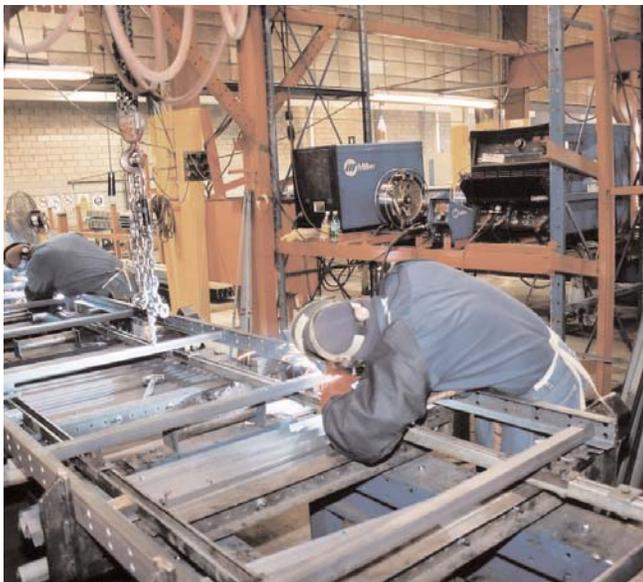
*Operators for Frazier Industrial weld cross beam sections for the company's storage rack systems. The welds have tight tolerances because they must meet strict standards for high seismic areas.*
