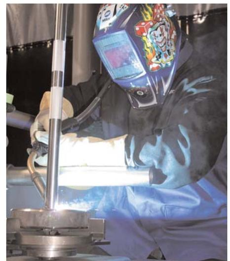
*An arm rest supports the operator’s arm while a turntable turns the part in place to eliminate a potential source of variability.*
