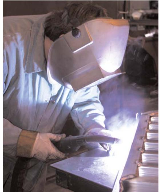
*By switching to the Millermatic 350P on its aluminum louver line, Greenheck saved 10 percent on rework and 25 percent on filler metal.*
