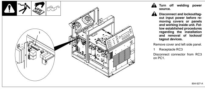
5. Connecting Programming Adapter To Control Board PC1
