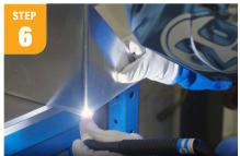
Tack weld each shelf to the back piece using a TIG welder. Consider installing a gas lens to the end of your TIG torch, which will help provide better gas coverage on the outer corners.
