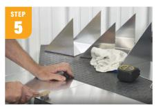
Peel the protective film off of the aluminum, then wire brush the areas you'll be welding and clean with acetone.
