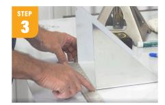
Once your shelves are cut and bent, measure each shelf to determine the width and height of the back piece. Mine ended up being 9.5/8'' wide x 52'' tall.
