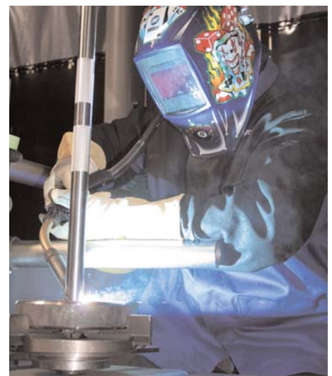
An arm rest supports the operator’s arm while a turntable turns the part in place to eliminate a potential source of variability.
