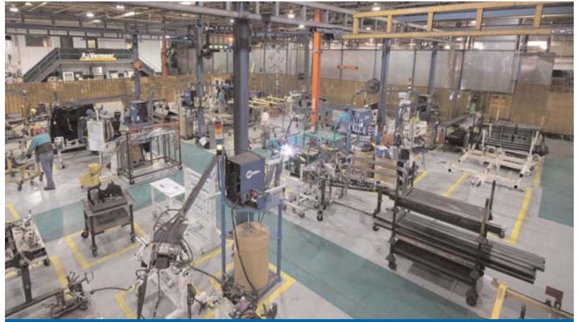
The welding area for Vermeer’s model line. Notice how boom-mounted feeders enable the operator to weld at several stations.
