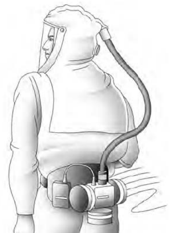
Hood Powered Air-Purifying Respirator (PAPR) APF= 25
