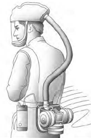
Loose-Fitting Powered Air-Purifying Respirator (PAPR) APF= 25
