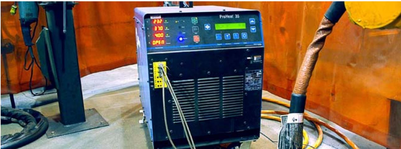
Hardened steel, which is used in high wear areas like base edges, doesn't like sudden changes. The same properties that make the steel wear better can also make it brittle. Because of this it needs to be carefully, and slowly, brought up to temperature prior to welding. Attention to detail is something we take pride-in and pre-heat is no exception.
