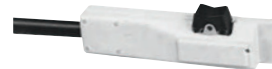
RMLS-14 (14-pin plug) 129337 Momentary- and maintained-contact rocker switch for contactor control. Push forward for maintained contact and backward for momentary contact. Includes 26.5-foot (8 m) cord with plug.
